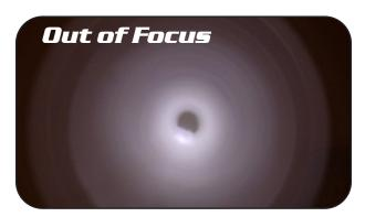
It is best to test your light against a blank wall in your house to fine tune the beam. If the head of the light is not screwed on tight enough, the beam will be uneven, rough, and could have a dark spot in the center.
