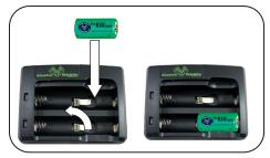
To place 16340 batteries in the Kill Light® Universal Charger, flip up the spring loaded contact plate in the center of the charging bay. Place the battery in the charging bay so it is held in place by the spring loaded contact plate. The charger includes A/C and 12 volt vehicle adapters for charging at home or on the go. The LED indicator will turn to red when charging and green when complete. It takes about one hour to charge the 16340 battery.
