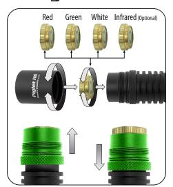
The Piglet HD™ has interchangeable LEDs. To change LEDs: First unscrew the head of the light by gripping the knurled ring and unscrewing the head. Slide the knurled ring collar towards the back to access the brass LED pill. Next, unscrew the brass LED pill from the body of the light. Then select the desired LED color and screw it into the body. Finally, slide the knurled ring collar towards the front of the light and tighten the head back onto the body.
